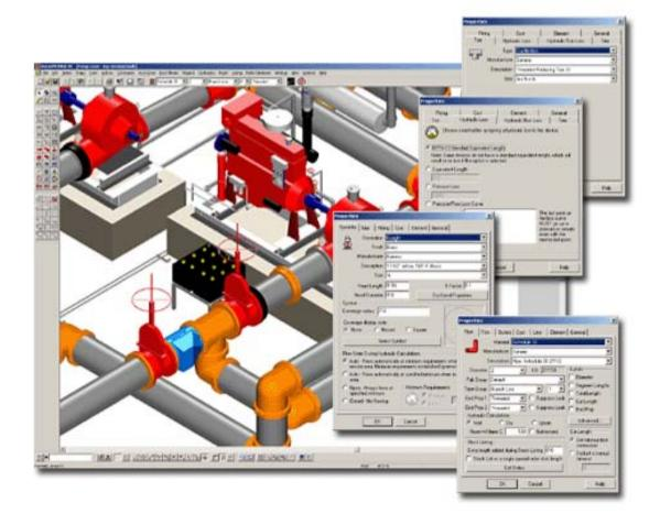
"Internally intelligent" elements emulate real world construction components in both appearance and performance taking on the exact characteristics of their real life counterparts. An AutoSPRINK VR pipe for example "knows" among other things, its size, pipe type and material, internal diameter, and Hazen/Williams C-factor; it also knows it has two pipe end-preps and must connect to another pipe, fitting or device
