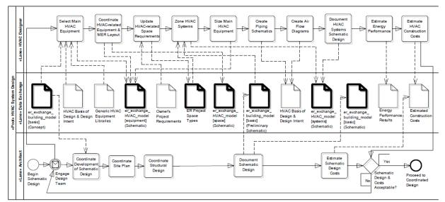
Figure 2. HVAC Schematic Design Process Model
