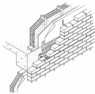
Exterior brick veneer/stud backup walls are defined in the following terms: type of brick and studs, stud spacing and bond. All systems include a back-up wall, a control joint every 20', a brick shelf every 12' of height, ties to the backup and the necessary damproofing, flashing and insulation.
