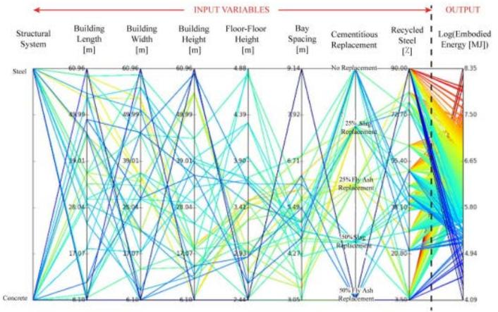
Figure 3: Parallel Coordinate Graph of Building Input Parameters and Total Embodied Energy.
