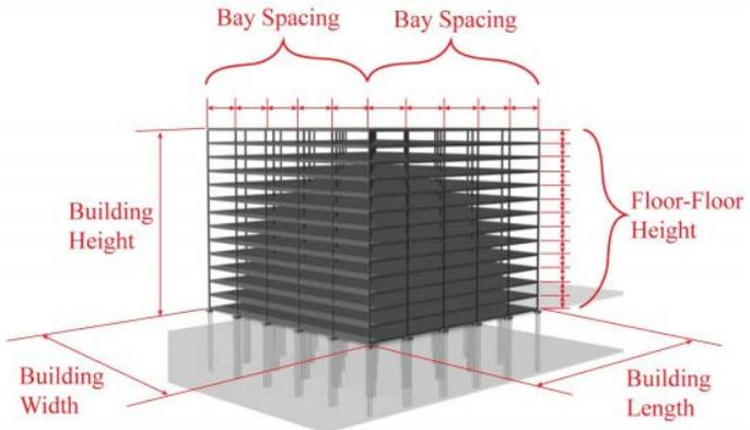
Figure 1: Geometric input parameters for embodied energy calculation.
