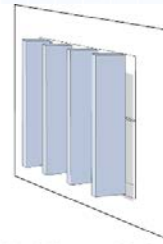
Vertical louvers or fins for east and especially west facades.
