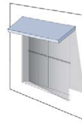
Slope it down for less projection.
