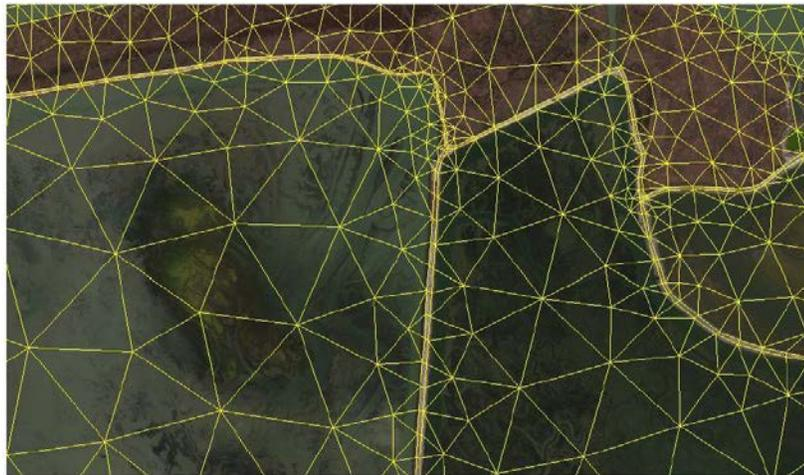
Figure 5.7 Detail of flexible model mesh resolution of embankment crests.
