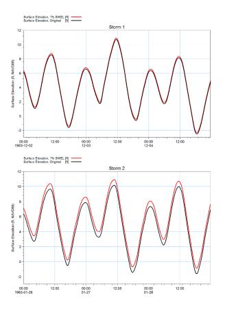
Figure Error! No text of specified style in document..1 Comparison of scaled time series for Storm 1 (upper), December 1983 and Storm 2 (lower), January 1983, at the center of the local model offshore boundary. The black line is the original time series from the regional model and the red line is scaled to the 1% level.
