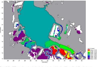
Figure 3.24 Difference in peak water levels (in meters) applying the 100-year South Bay discharges minus baseline simulation. December 1983 storm.
