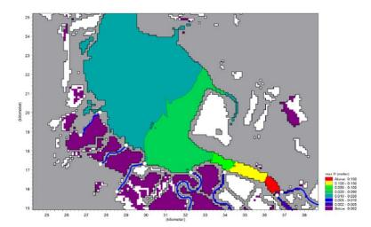
Figure 3.23 Difference in peak water level, (in meters) applying the 100-year Coyote Creek discharge minus baseline simulation. January 1983 storm.
