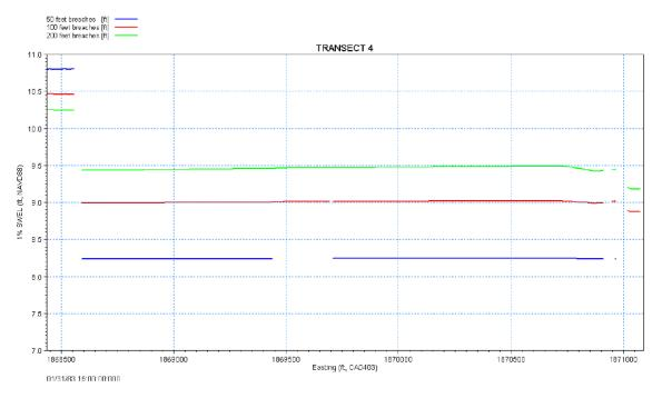
Figure 4.14 Approximate 1% SWEL along Transect 4 for the 3 breach widths. The blue line is 50 foot breach widths, red is 100 foot breach widths, and green is 200 foot breach widths.
