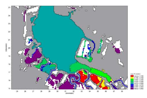
Figure 3.24 Difference in peak water levels (in meters) applying the 100-year South Bay discharges minus baseline simulation. December 1983 storm.
