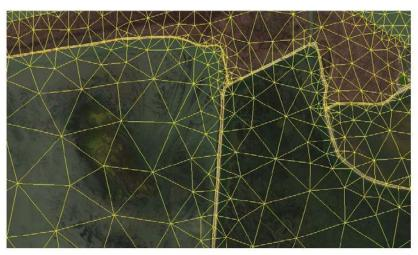
Figure 5.7 Detail of flexible model mesh resolution of embankment crests.
