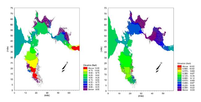
Figure 4.5 Maps of model predicted maximum water surface elevation for a high water event in January 1983. The figure on the left is the model with levees included, and the figure on the right is the model with all levees completely removed.
