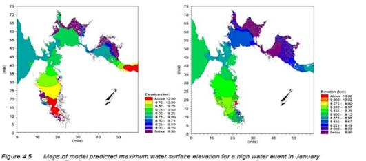
ure 4.5 Maps of model predicted maximum water surface elevation for a high water event in Januai 1983. The figure on the left is the model with levees included, and the figure on the right is the model with all levees completely removed.
