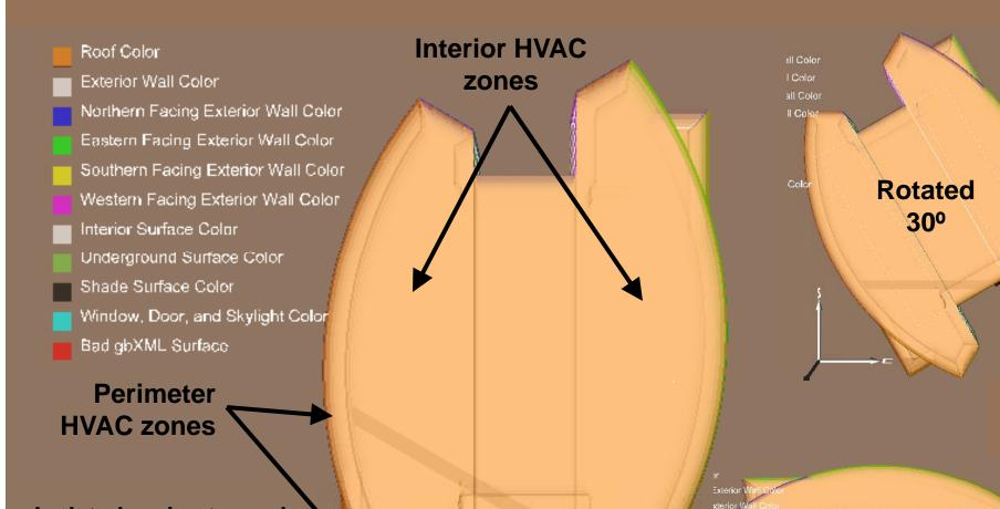
Isolated perimeter and interior HVAC zones provide thermal heat gain & heat loss predictions on the building
