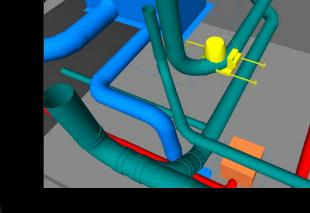
Would have required moving of light fixture with adverse effect on architecture.
