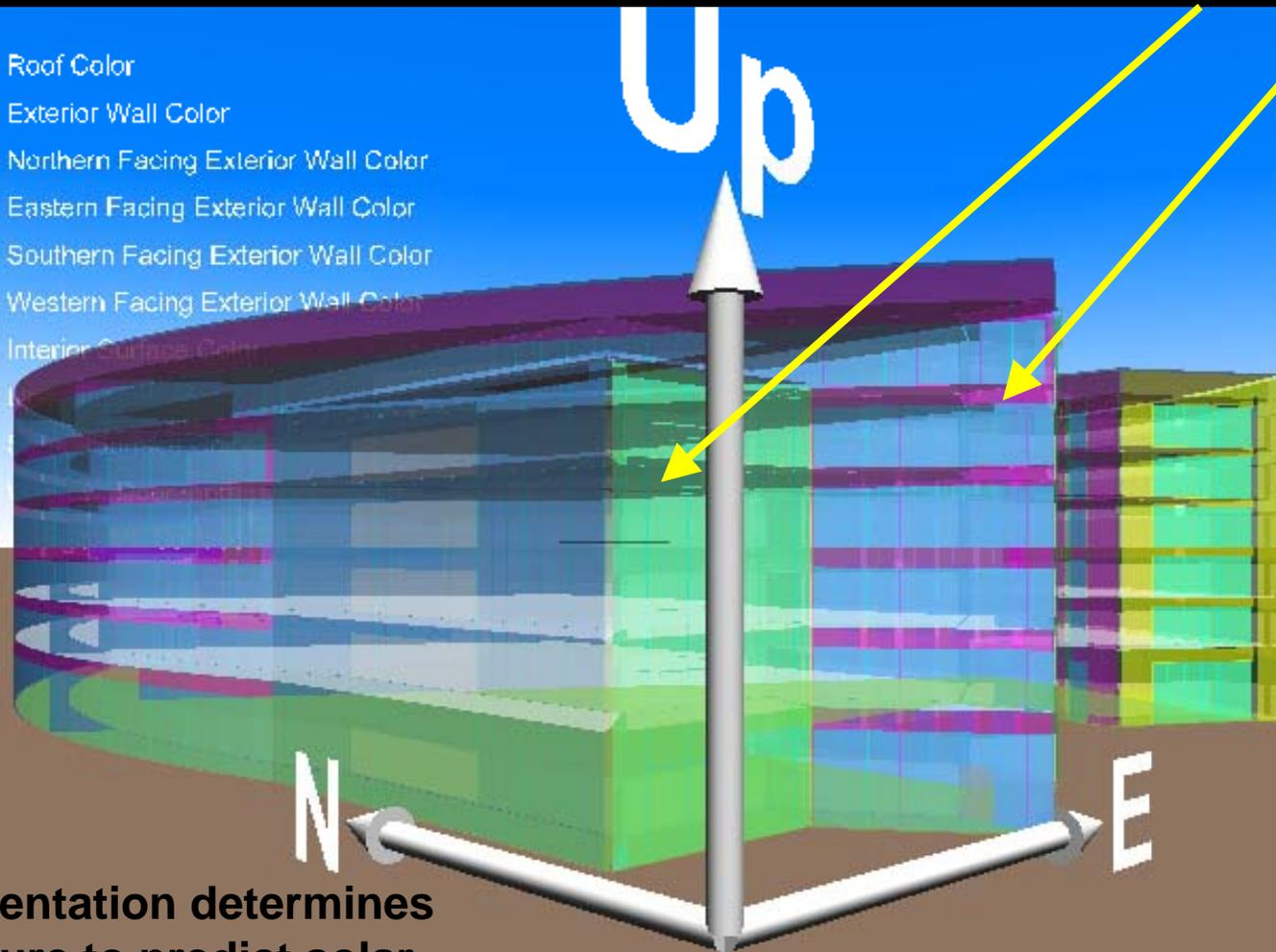
**Building orientation determines solar exposure to predict solar heat gain**
