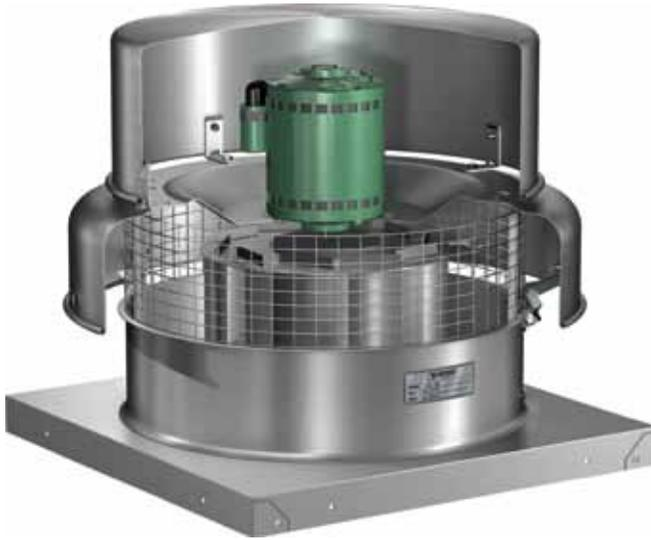
Spun aluminum downblast exhaust fans shall be direct drive type. These fans are specifically designed for roof mounted applications exhausting relatively clean air. Performance capabilities range up to 6,640 cfm (11,281 m<sup>3</sup>/hr) and 1 in. wg (249 Pa) of static pressure. The maximum continuous operating temperature shall be 180°F (82°C). Model G fans are available in 20 sizes with nominal wheel diameters ranging from 7 to 20 inches (178 to 457 mm) (060-203 unit sizes).
