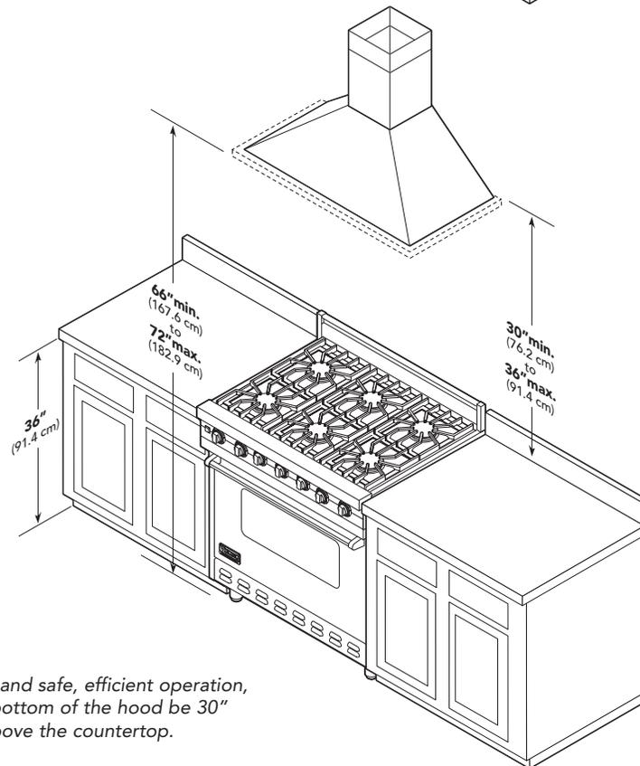
**Note:** For best performance and safe, efficient operation, it is recommended that the bottom of the hood be 30" (76.2 cm) to 33" (83.8 cm) above the countertop.
